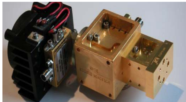
Fig. 1: A THz source consisting of a low frequency coaxial input, an integrated doubler/amplifier, a quadrupler and two triplers. It has generated up to 25 microwatts in the WR-0.65 waveguide band. Total length is six-inches. No mechanical tuners are used.
